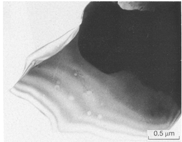
Figure 9 TEM image of the iridium coating on the polished surface of C/C composite after heat treatment, showing crystalline grains with very small voids.
